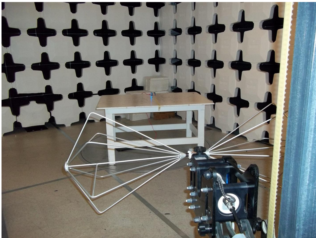
Figure 3. Radiated Emissions Test Configuration (30-200 MHz)
