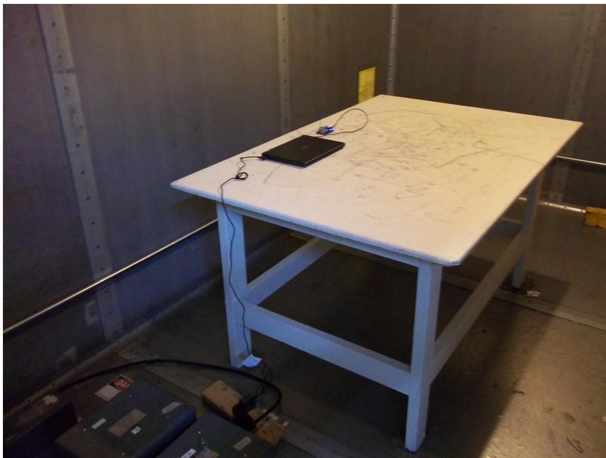
Figure 7. Power Line Conducted Emissions Test Configuration
