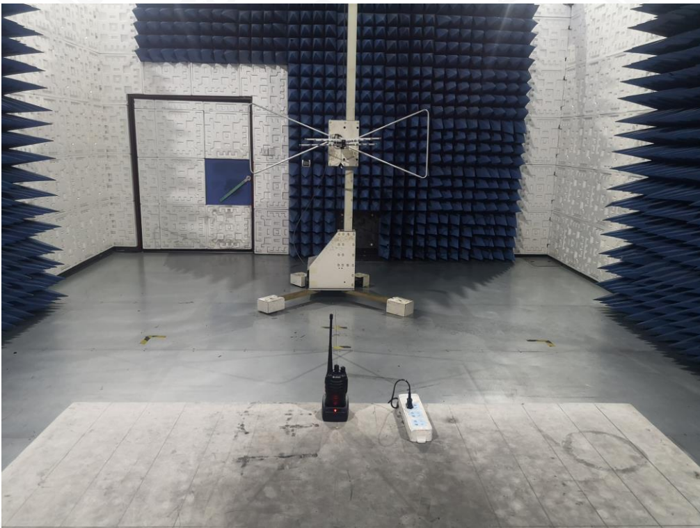
RADIATED EMISSION TEST SETUP-BELOW 1GHZ
