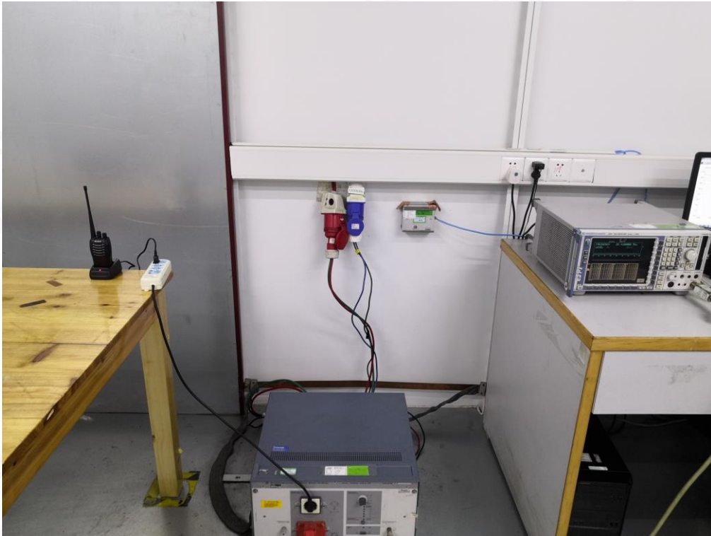
RADIATED EMISSION TEST SETUP-BELOW 1GHZ
