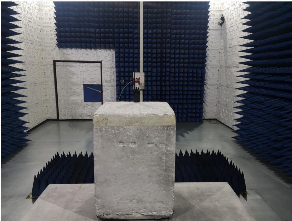
RADIATED EMISSION ABOVE 1G TEST SETUP
