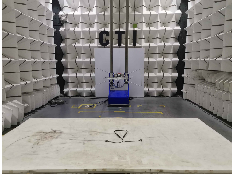
Radiated spurious emission Test Setup-1(Below 1GHz)
