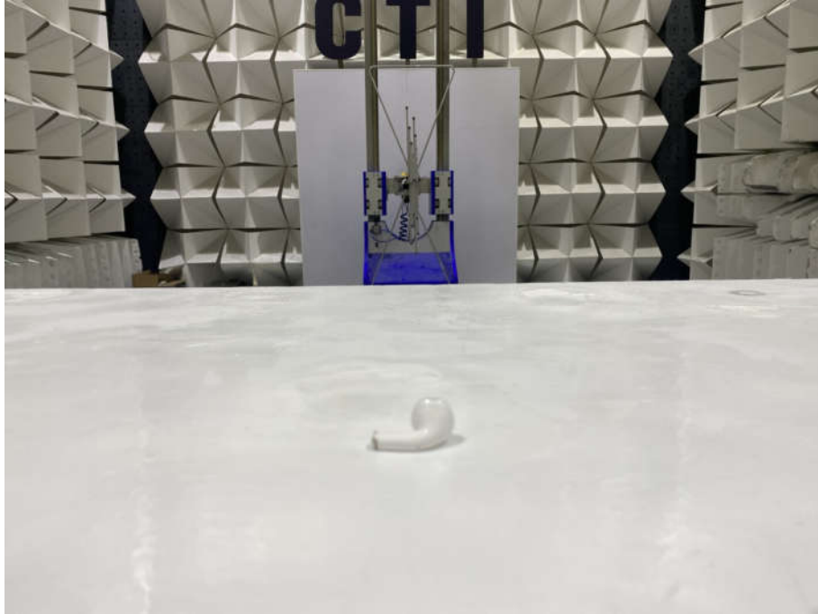
Radiated spurious emission Test Setup-1(Below 1GHz) Ear L
