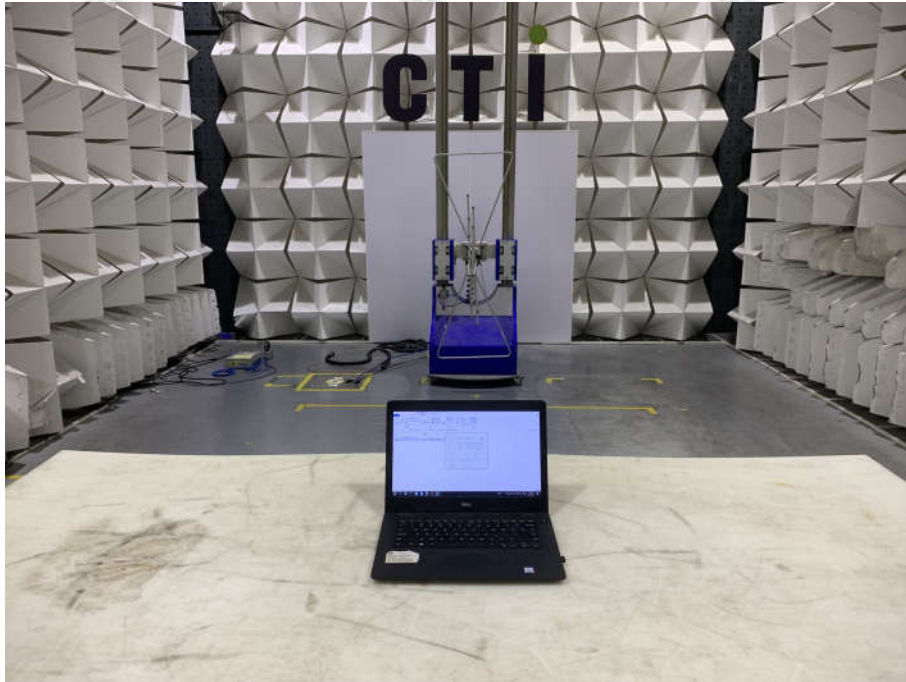
Radiated spurious emission Test Setup-1(Below 1GHz)
