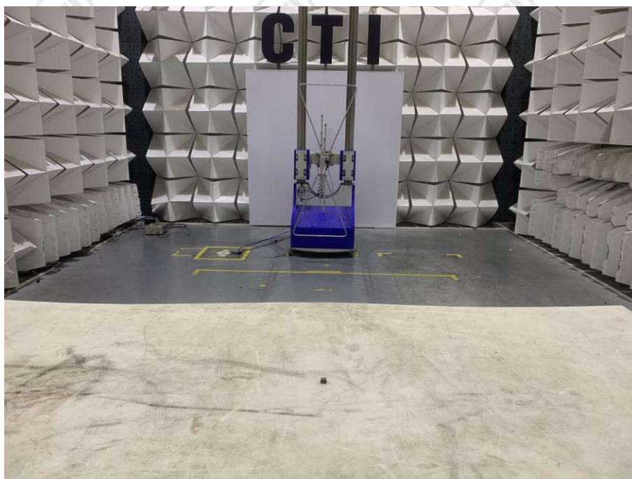
Radiated spurious emission Test Setup-1(Below 1GHz)
