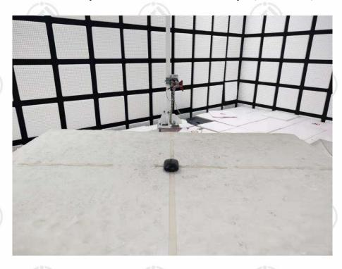
Radiated spurious emission Test Setup-2(Above 1GHz)
