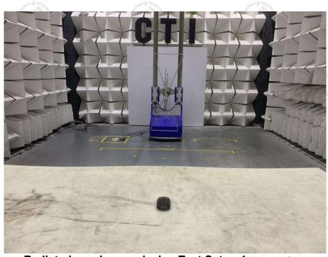
Radiated spurious emission Test Setup-1(Below 1GHz)
