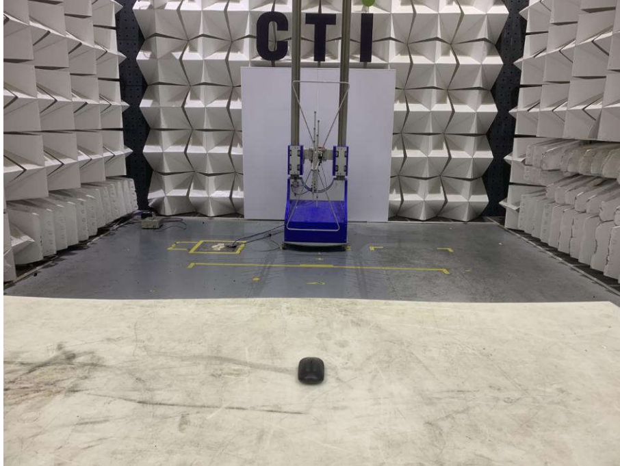
Radiated spurious emission Test Setup-1(Below 1GHz)
