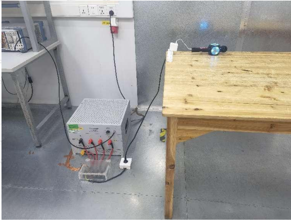
Photo of Conducted Emission Measurement
