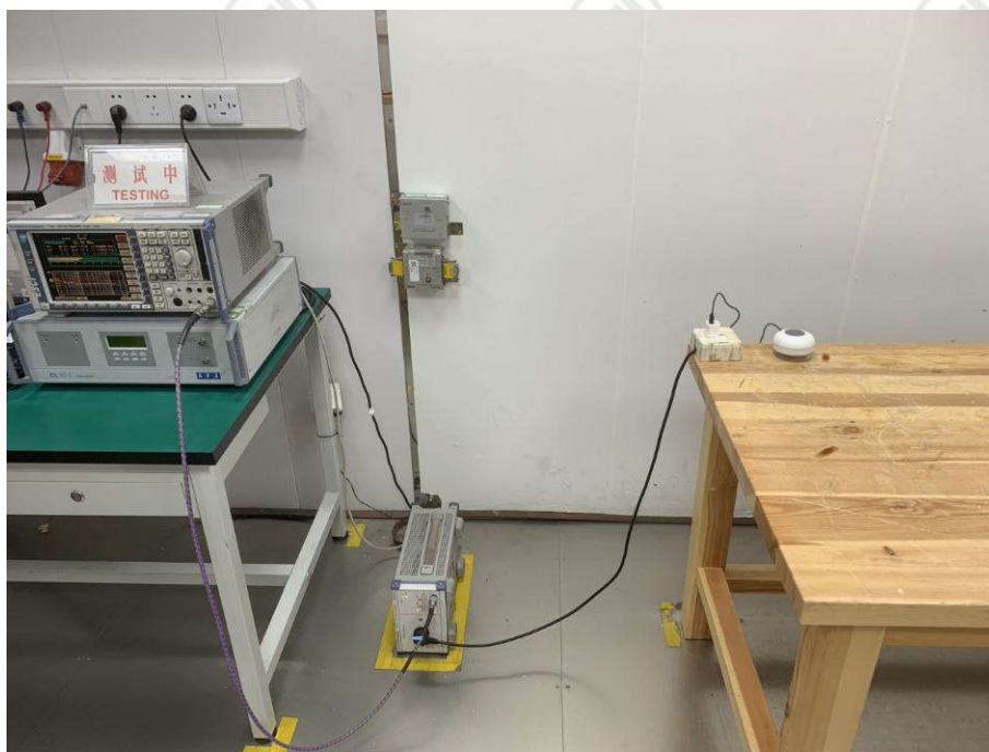
CONDUCTED EMISSION TEST SETUP
