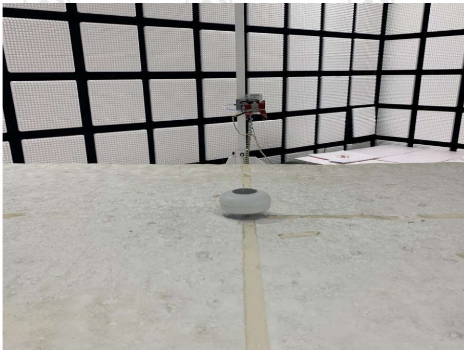
Radiated spurious emission Test Setup-2(Above 1GHz)
