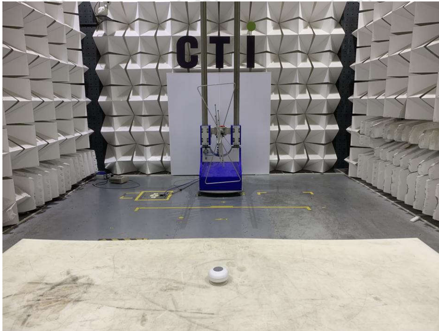
Radiated spurious emission Test Setup-1(Below 1GHz)
