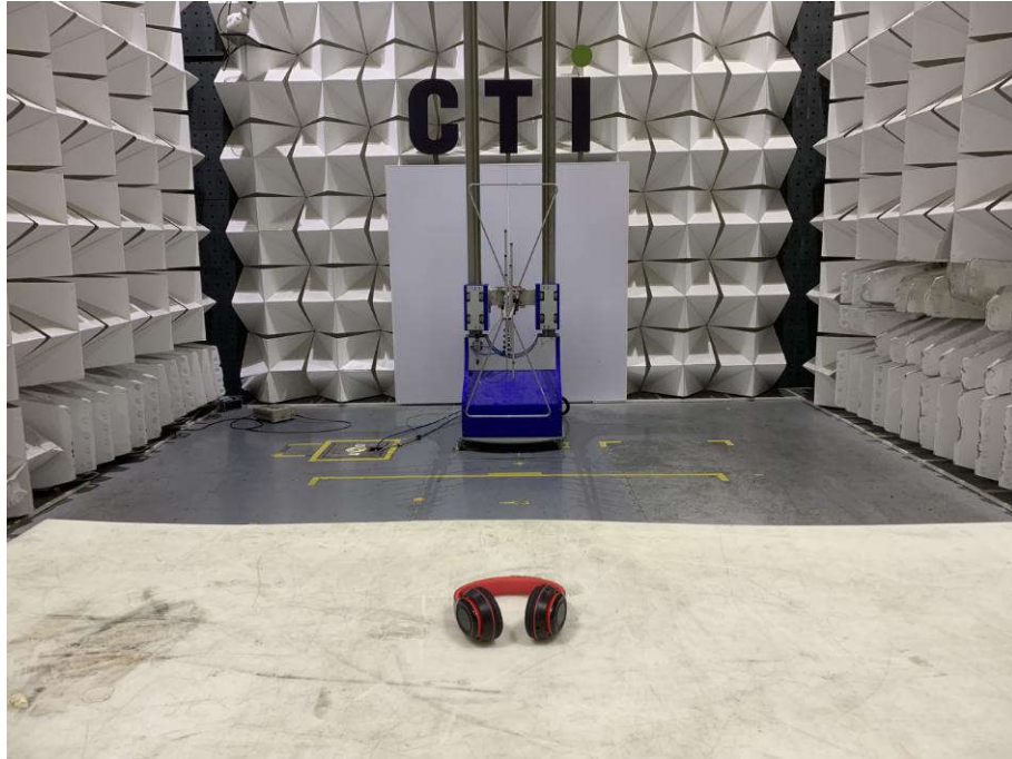
Radiated spurious emission Test Setup-1(Below 1GHz)
