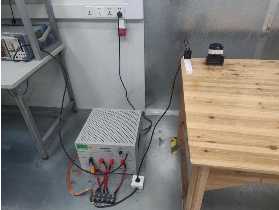
Photo of Conducted Emission Measurement
