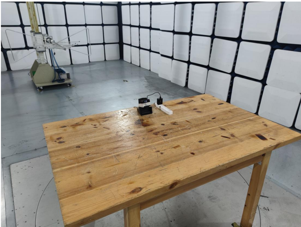
Photo of Radiation Emission Test
