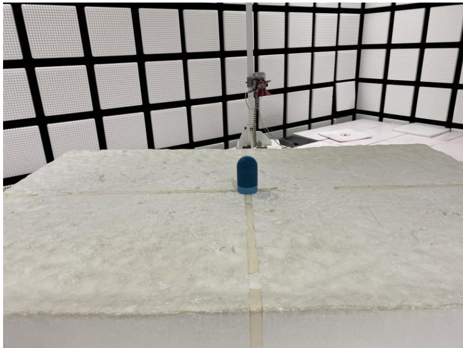
Radiated spurious emission Test Setup-2(Above 1GHz)
