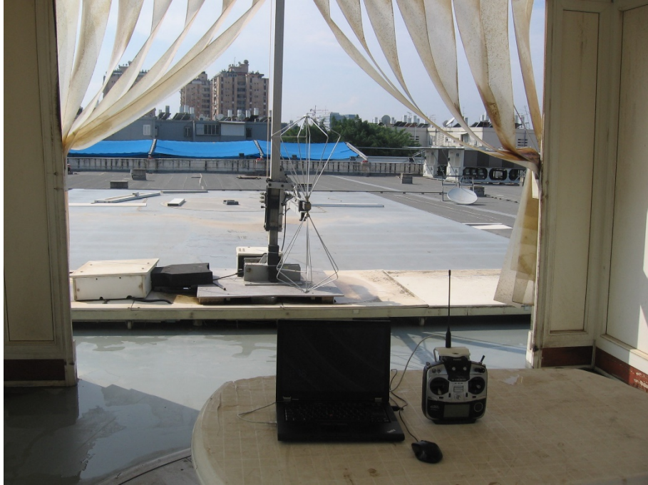
Figure 6. Radiated Emission Test, 30-200MHz
