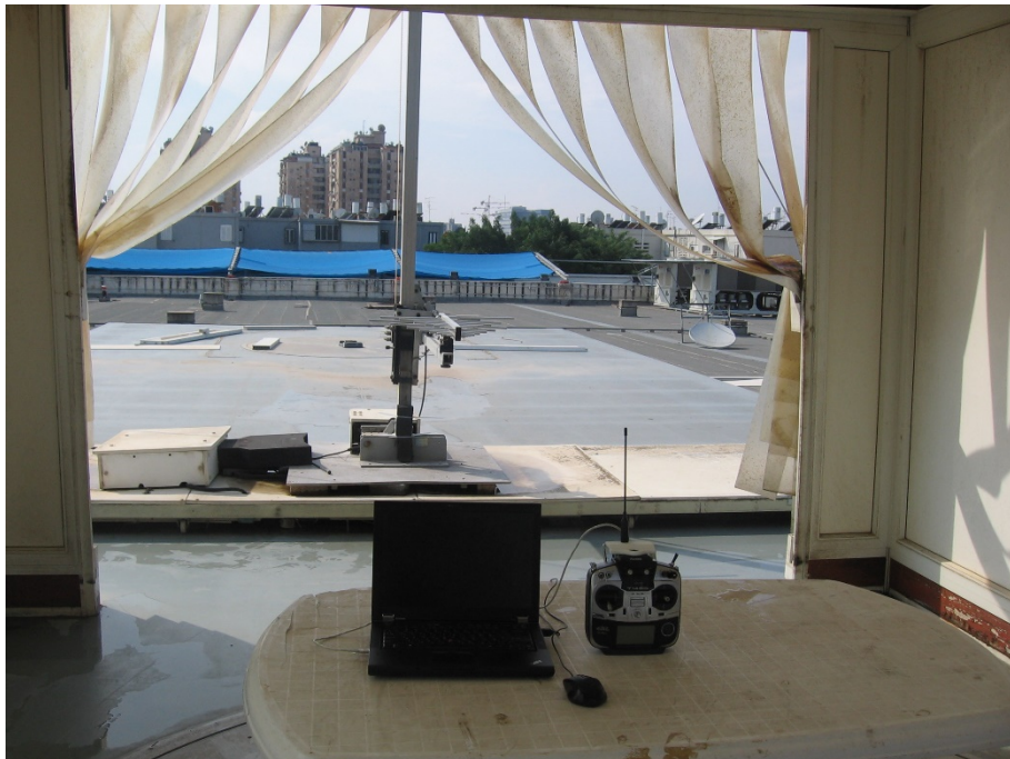
Figure 7. Radiated Emission Test, 200-1000MHz
