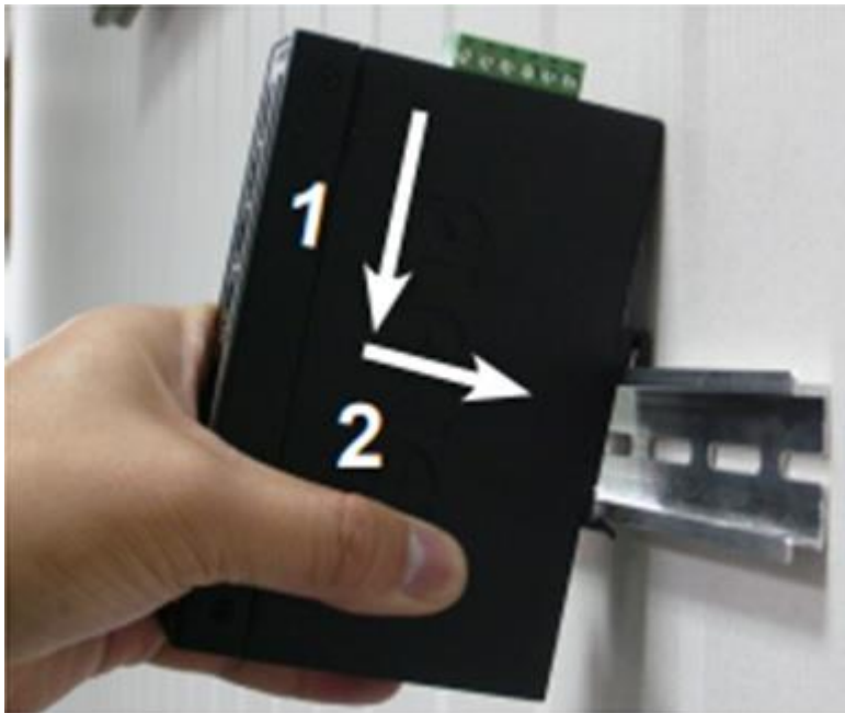
Figure 25 Mount the POE-162 Injector on the DIN mounting rail
