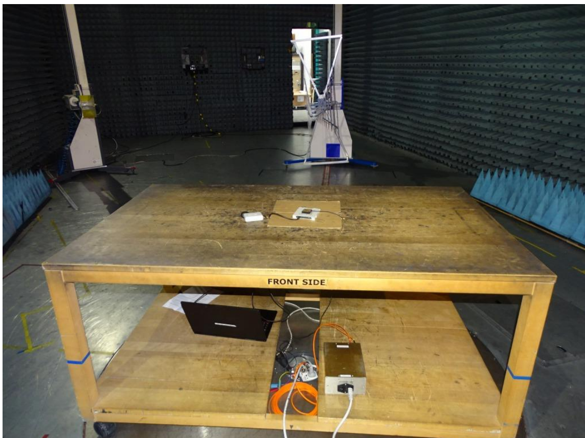
Photo 2: Test setup for radiated measurements below 1 GHz
