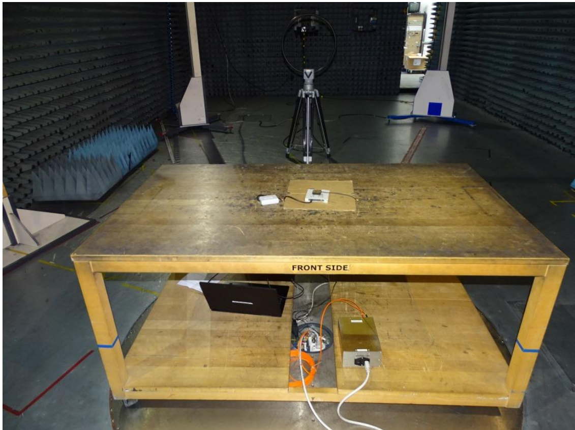
Photo 1: Test setup for radiated measurements below 30 MHz
