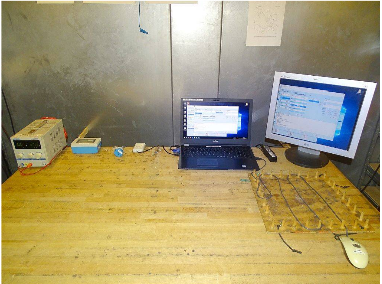
Photo 4: Test setup for conducted measurements (AC Port power line), EUT supplied by and connected to AC Mains via laboratory power supply, intentional radiator §15, ANSI C63.10
