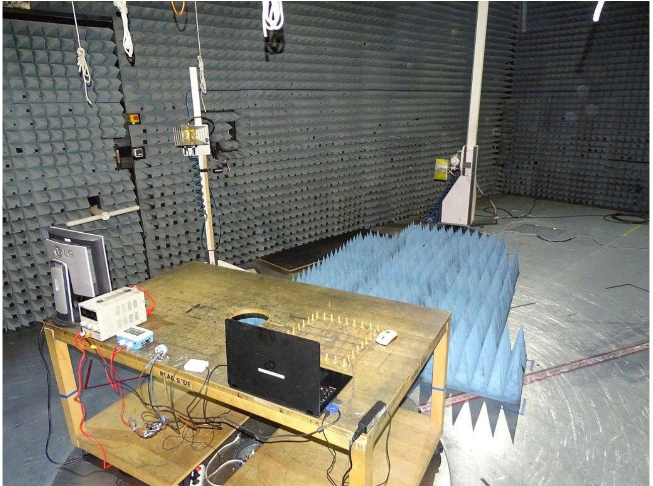
Photo 8: Test setup for radiated measurements (computer peripheral setup, EUT connected to AC Mains via laboratory power supply, fully-anechoic chamber, 1-13 GHz, unintentional radiator §15.109, ANSI C63.4)
