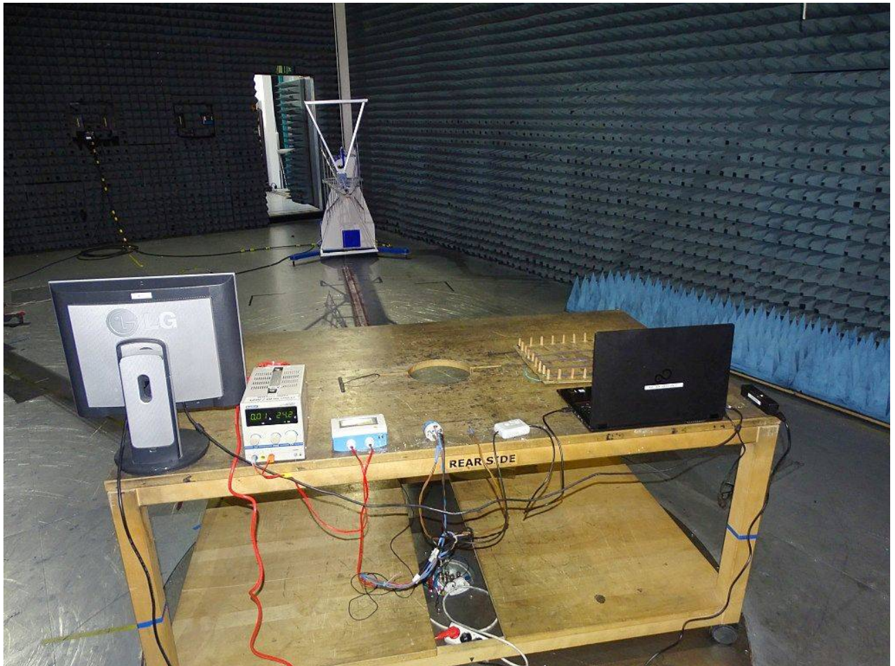
Photo 7: Test setup for radiated measurements (computer peripheral setup, EUT connected to AC Mains via laboratory power supply, semi-anechoic chamber, 30 MHz to 1 GHz, unintentional radiator §15.109, ANSI C63.4)
