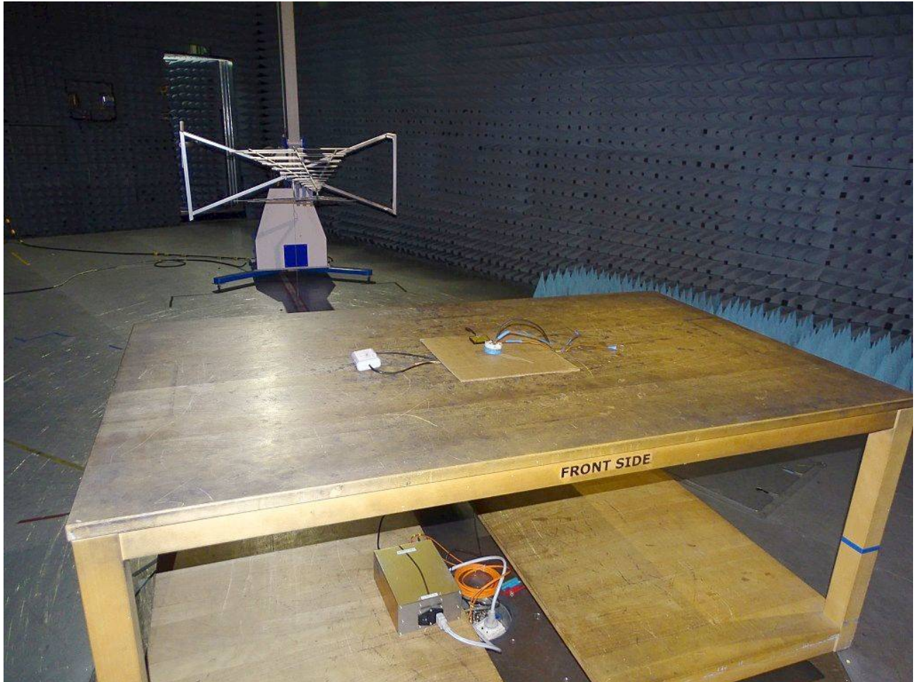
Photo 2: Test setup for radiated measurements (Enclosure, semi-anechoic chamber, 30 MHz to 1 GHz, intentional radiator §15, ANSI C63.10)
