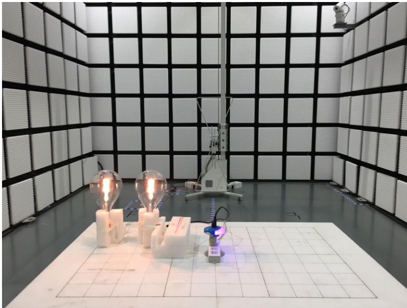
Fig.4 Radiated emission setup photo(30MHz-1GHz)
