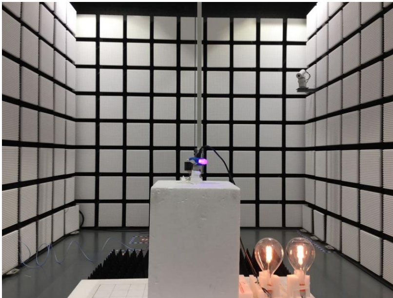
Fig.6 Radiated emission setup photo(Above 1GHz)
