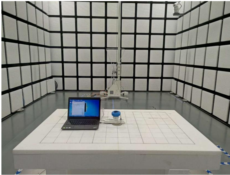
Fig.3 Radiated emission setup photo(30MHz-1GHz)
