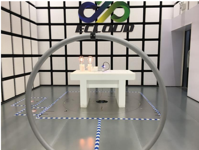
Fig.2 Radiated emission setup photo(Below 30MHz)
