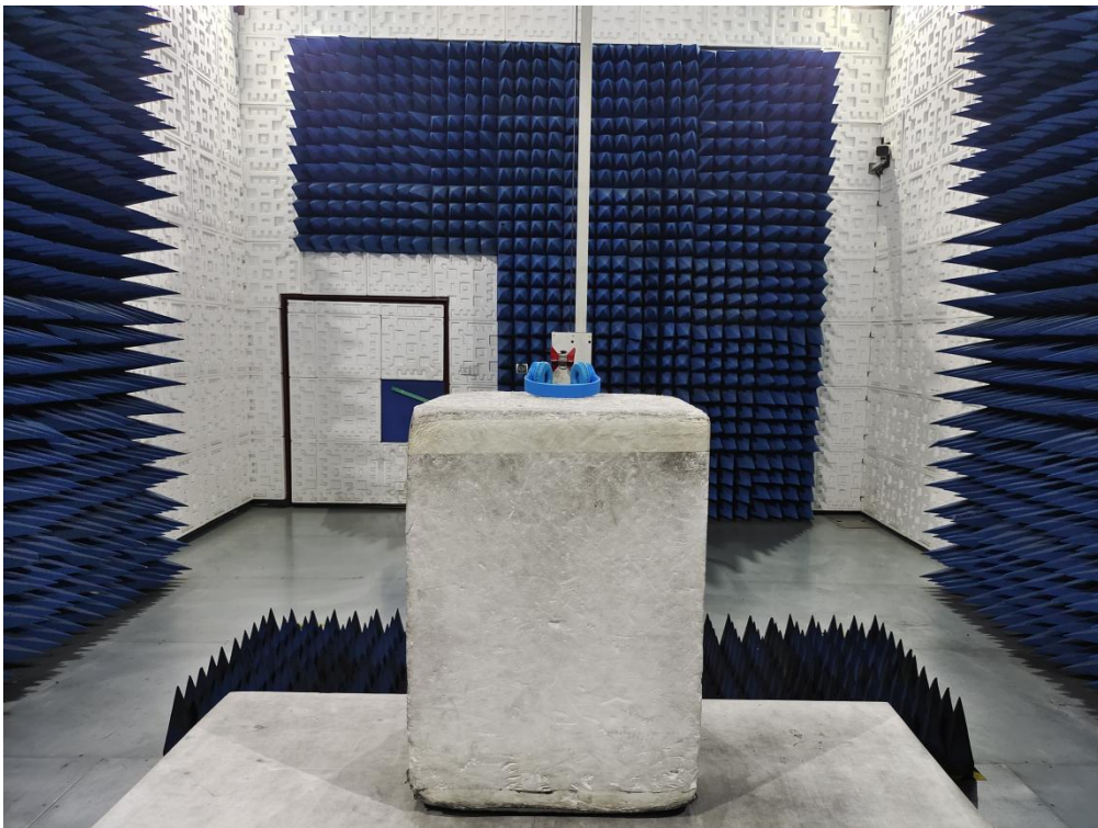
RADIATED EMISSION TEST SETUP ABOVE 1GHz
