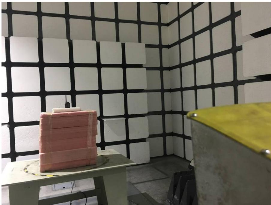
Radiated Emissions View (Above 1 GHz)
