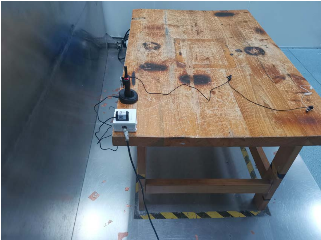
Conducted Emissions Side View--Adapter 2#
