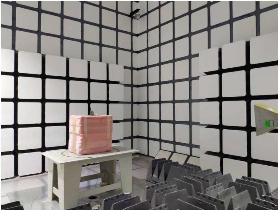
Radiated Emissions View (Above 1 GHz)
