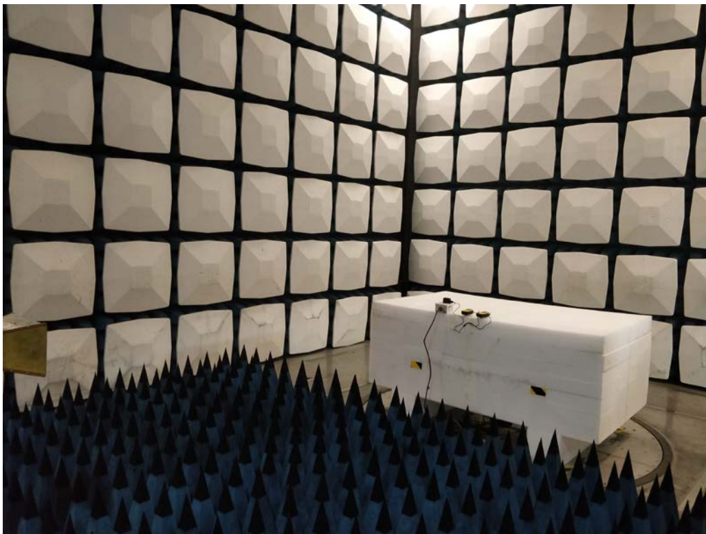
Radiated Emission Above 1GHz Rear View
