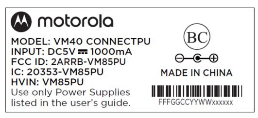
The label shown shall be permanently affixed at a conspicuous location on the device and be readily visible to the user at the time purchase (Labeling requirements per 2.925)
