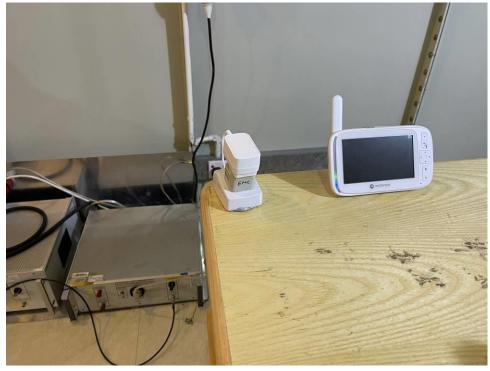
Radiated Emissions (30MHz-1GHz) Test Setup
