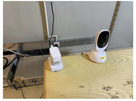
Radiated Emissions (30MHz-1GHz) Test Setup
