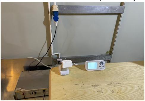
Radiated Emissions (30MHz-1GHz) Test Setup
