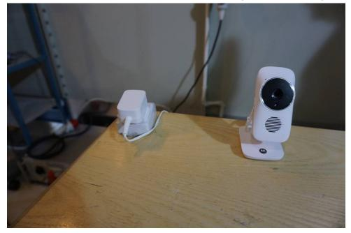
Radiated Emissions (30MHz-1GHz) Test Setup
