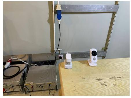
Radiated Emissions (30MHz-1GHz) Test Setup
