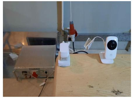
Radiated Emissions (30MHz-1GHz) Test Setup
