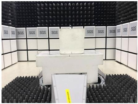
**Conducted RF Output Power Test Setup**
