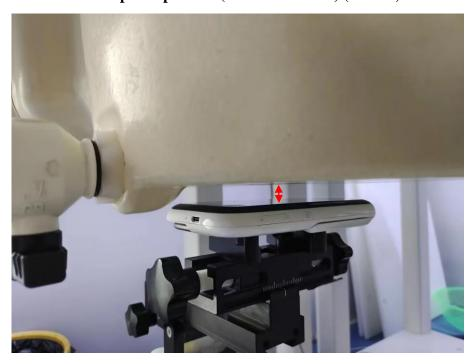
Face Up Setup Photo (Antenna Open) (10 mm)
