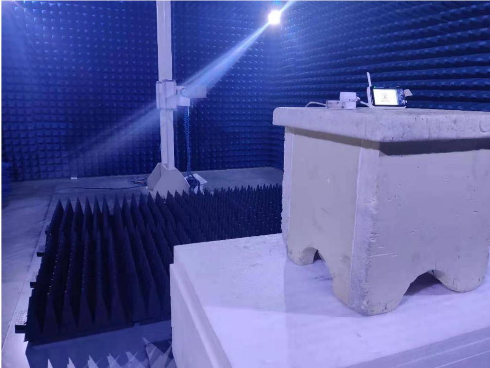
Photo of Radiated Emission Measurement (Above 1G)
