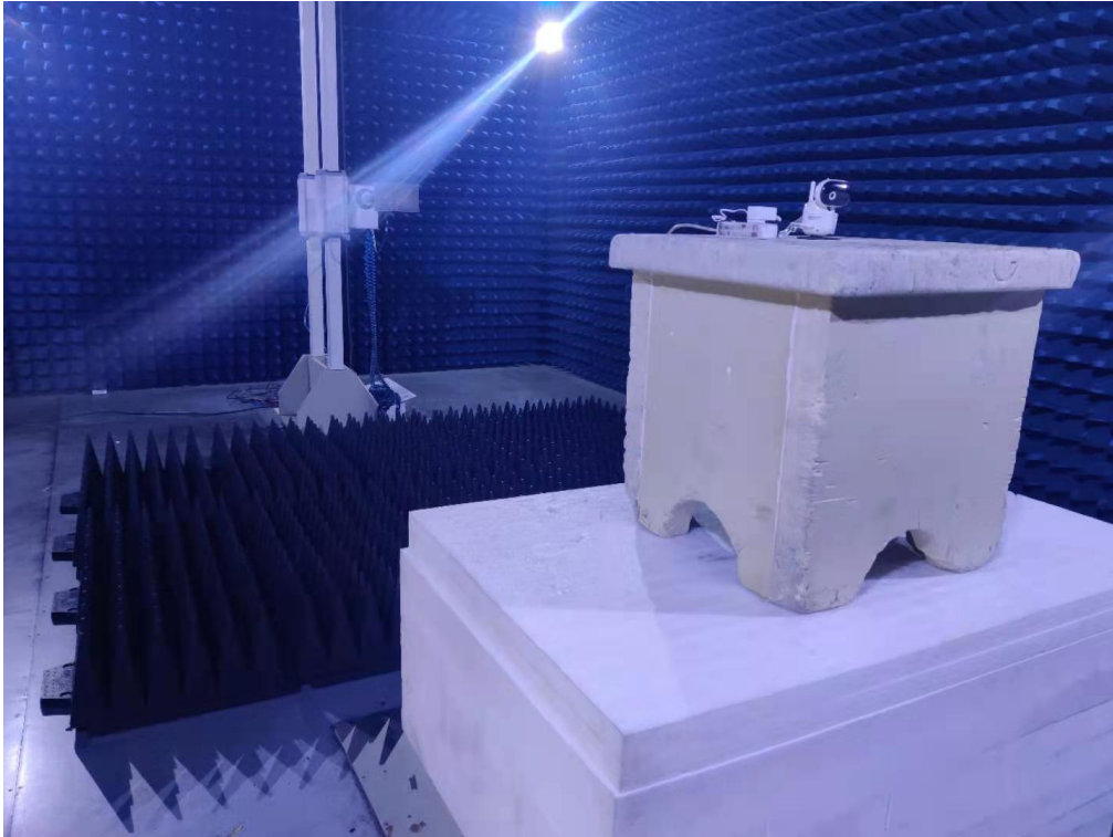
Photo of Radiated Emission Measurement (Above 1G)
