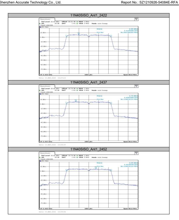
Appendix C: Maximum conducted Peak output power Test Result
