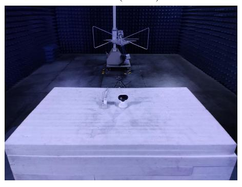
Photo of Radiated Emission Measurement (Above 1G)
