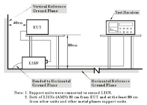
The setup of EUT is according with per ANSI C63.10-2013 measurement procedure. The specification used was with the FCC Part 15.207 & RSS-Gen limits.
