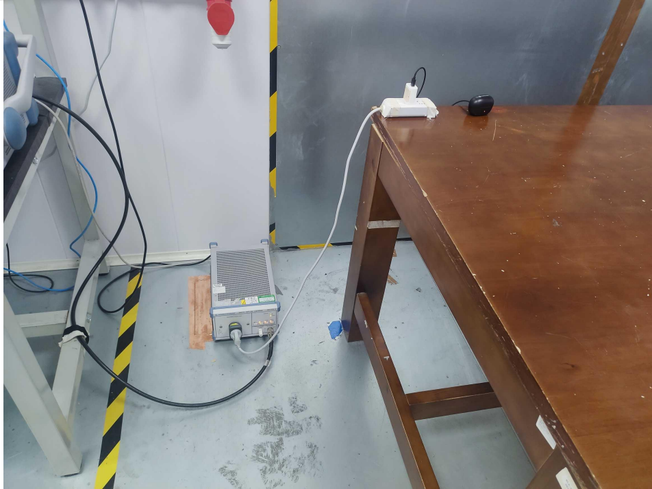
Conducted emissions at AC power line (150kHz-30MHz)
