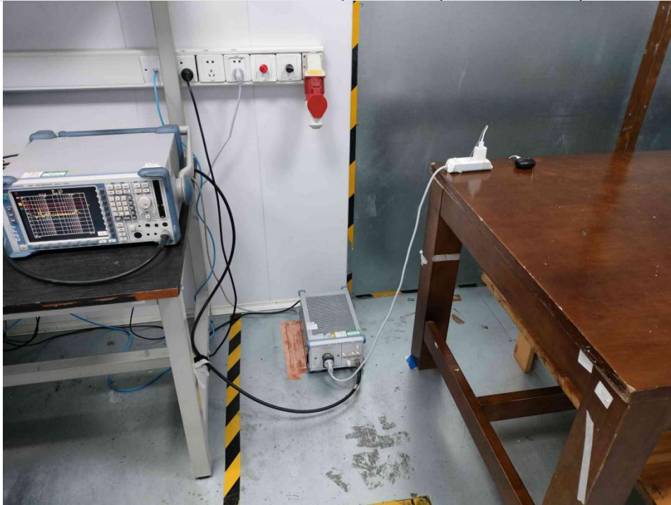
Conducted emissions at AC power line (150kHz-30MHz)
