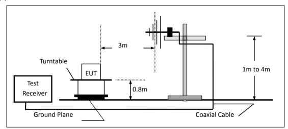
(c) For radiated emissions above 1000MHz
