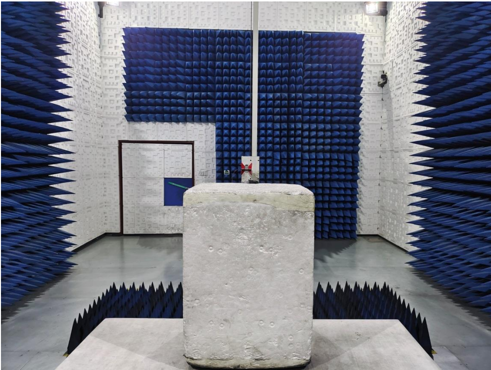
RADIATED EMISSION TEST SETUP ABOVE 1GHz
