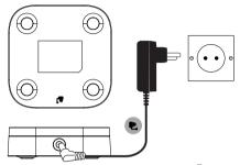
Plug the AC power adaptor into the socket marked L on the rear of the charger and plug the other end into the AC power outlet. Switch on the AC power.
