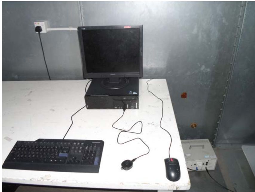
Measurement of Conducted Emission Test Set Up
