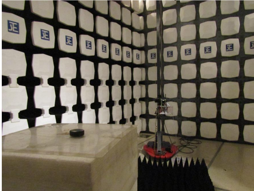
Measurement of Conducted Emission Test Set Up
