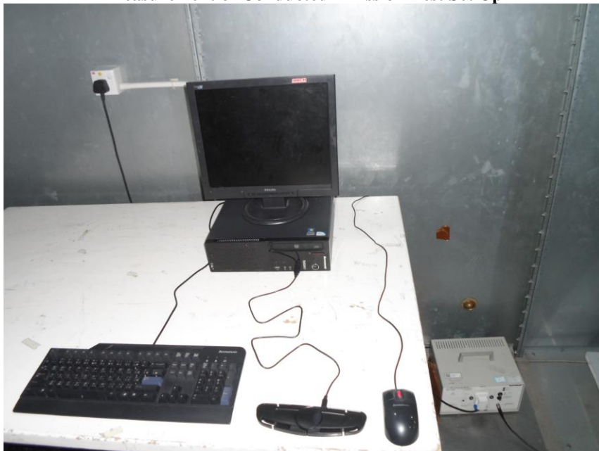
Measurement of Conducted Emission Test Set Up
