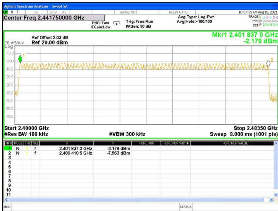
Hopping No. NVNT 3-DH1 2441MHz Ant1
