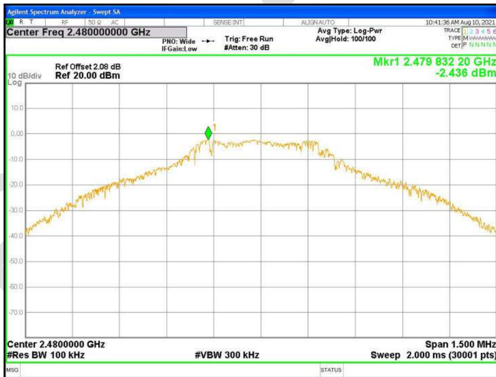
Tx. Spurious NVNT 1-DH1 2480MHz Ant1 Emission
