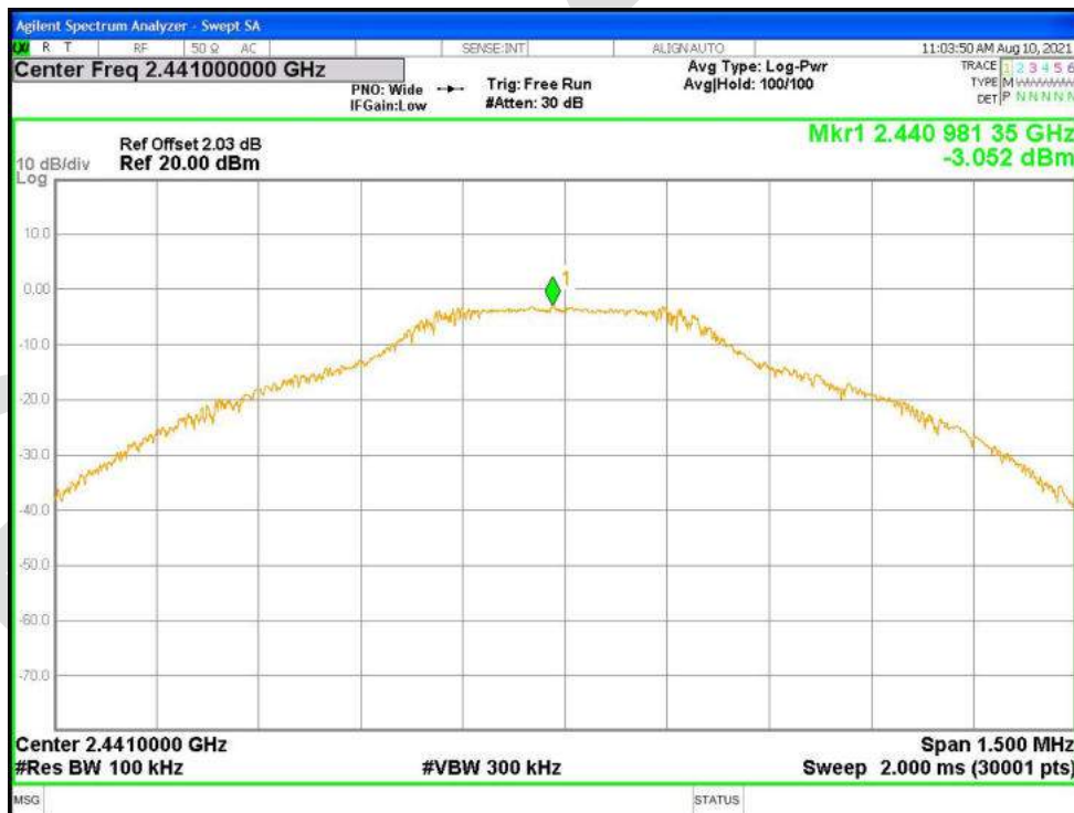
Tx. Spurious NVNT 3-DH1 2441MHz Ant1 Emission
