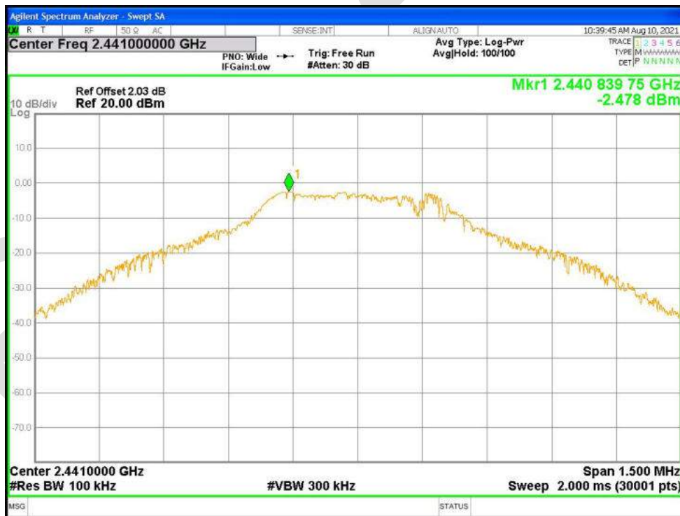
Tx. Spurious NVNT 1-DH1 2441MHz Ant1 Emission
