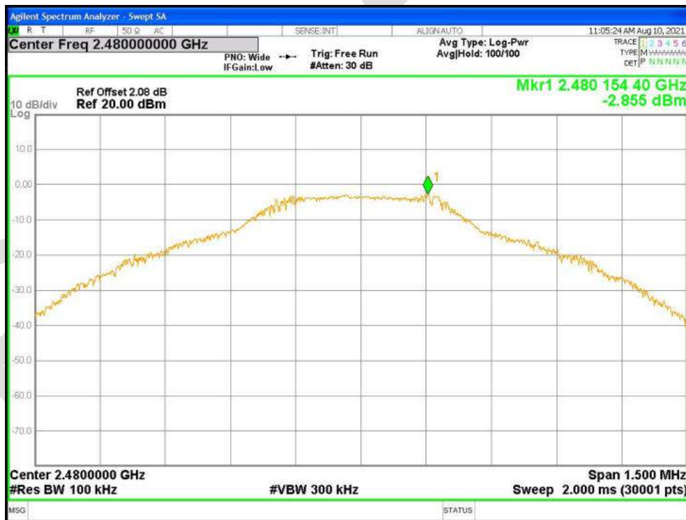
Tx. Spurious NVNT 3-DH1 2480MHz Ant1 Emission
