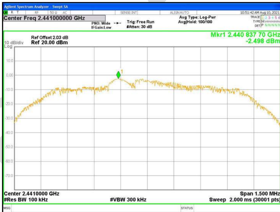
Tx. Spurious NVNT 2-DH1 2441MHz Ant1 Emission
