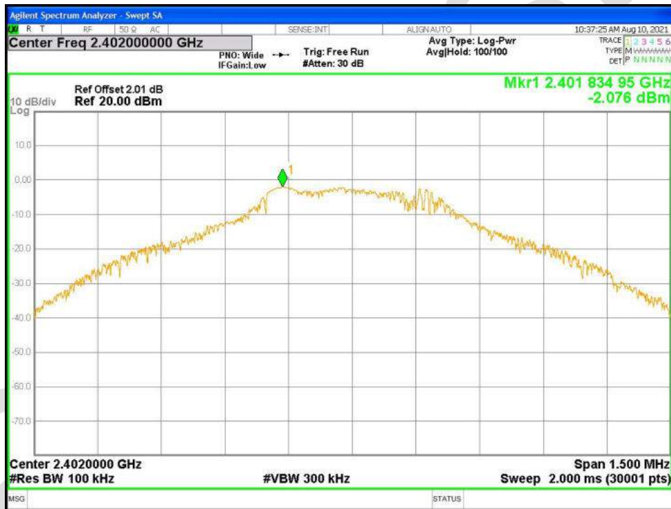
Tx. Spurious NVNT 1-DH1 2402MHz Ant1 Emission
