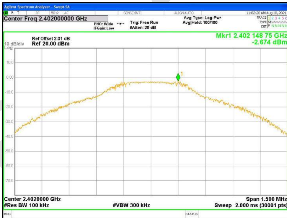
Tx. Spurious NVNT 3-DH1 2402MHz Ant1 Emission
