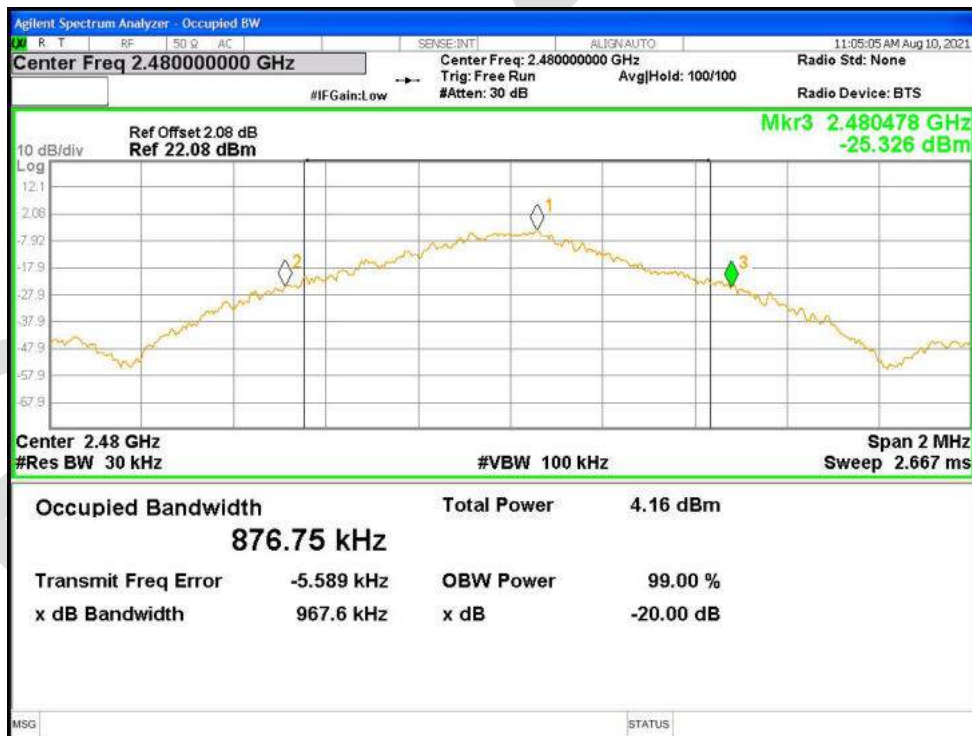
-20dB Bandwidth NVNT 3-DH1 2480MHz Ant1
