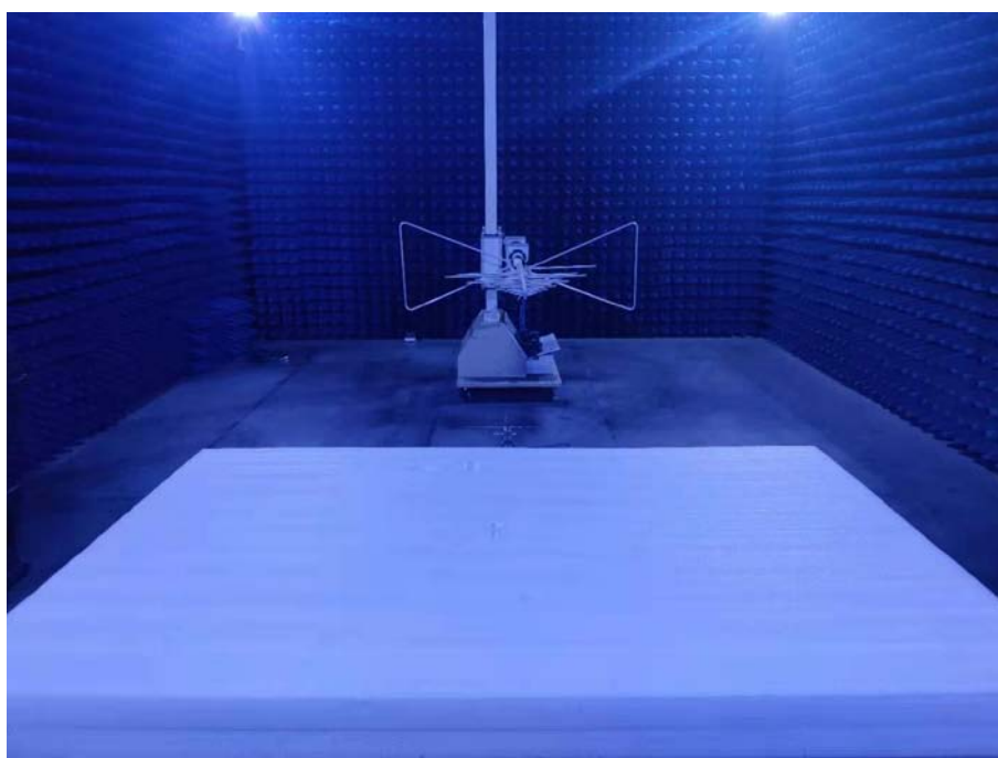
Photo of Radiated Emission Measurement (Below 1G)
