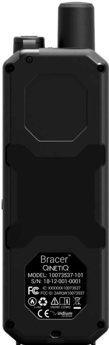
Location of Product Label on rear of case of Bracer PTT Handset
