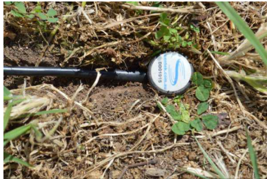
Figure 4 Properly installed probe
