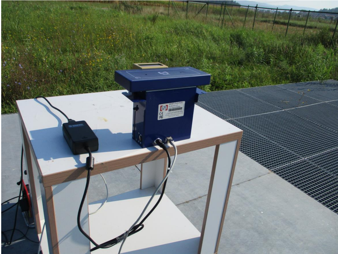
Figure 11: Radiated emission tests - OATS
