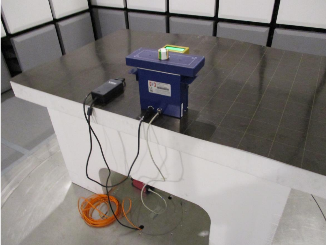
Figure 7: Radiated emission test from 200 MHz to 1 GHz
