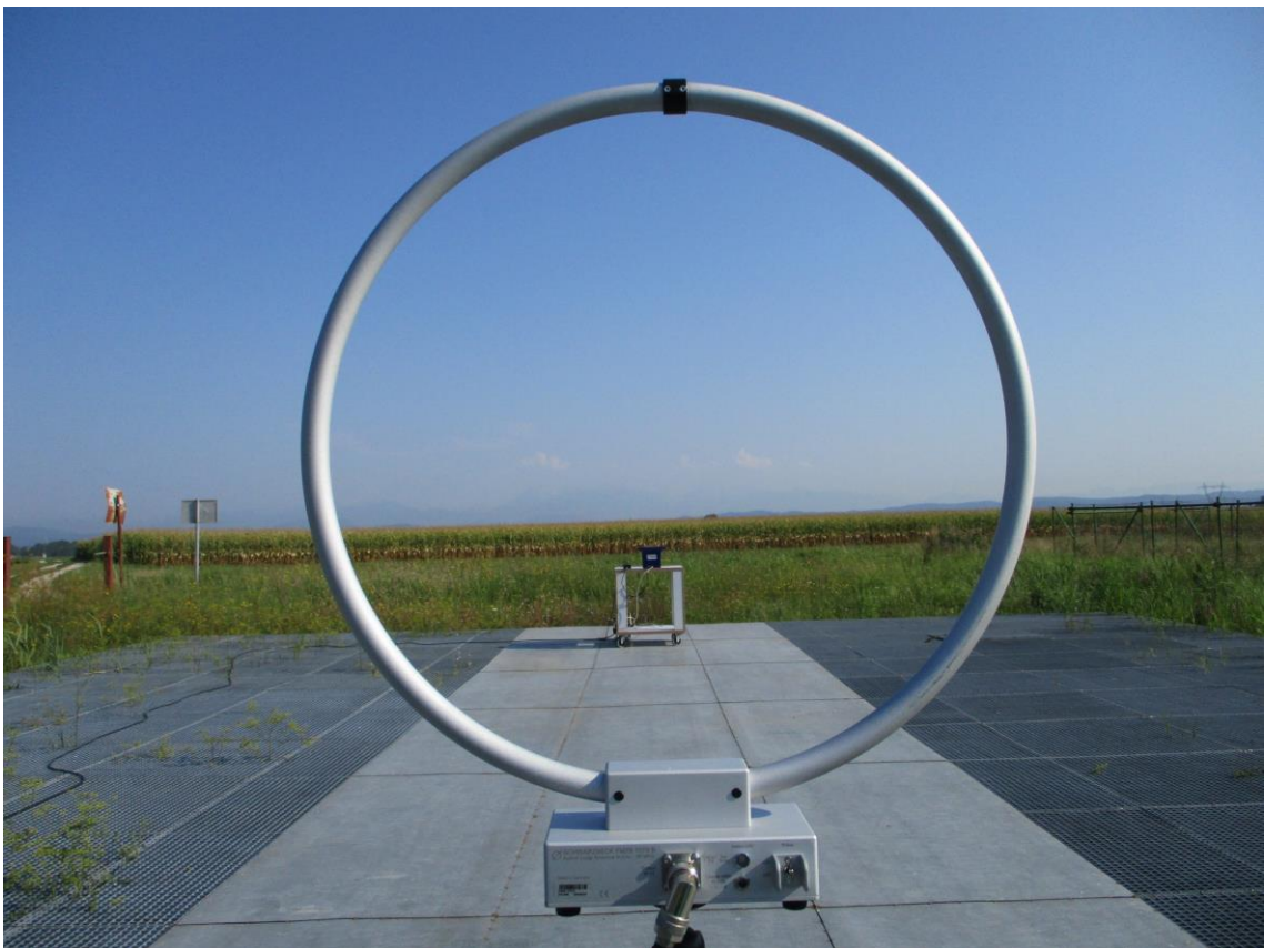
Figure 10: Radiated emission tests - OATS
