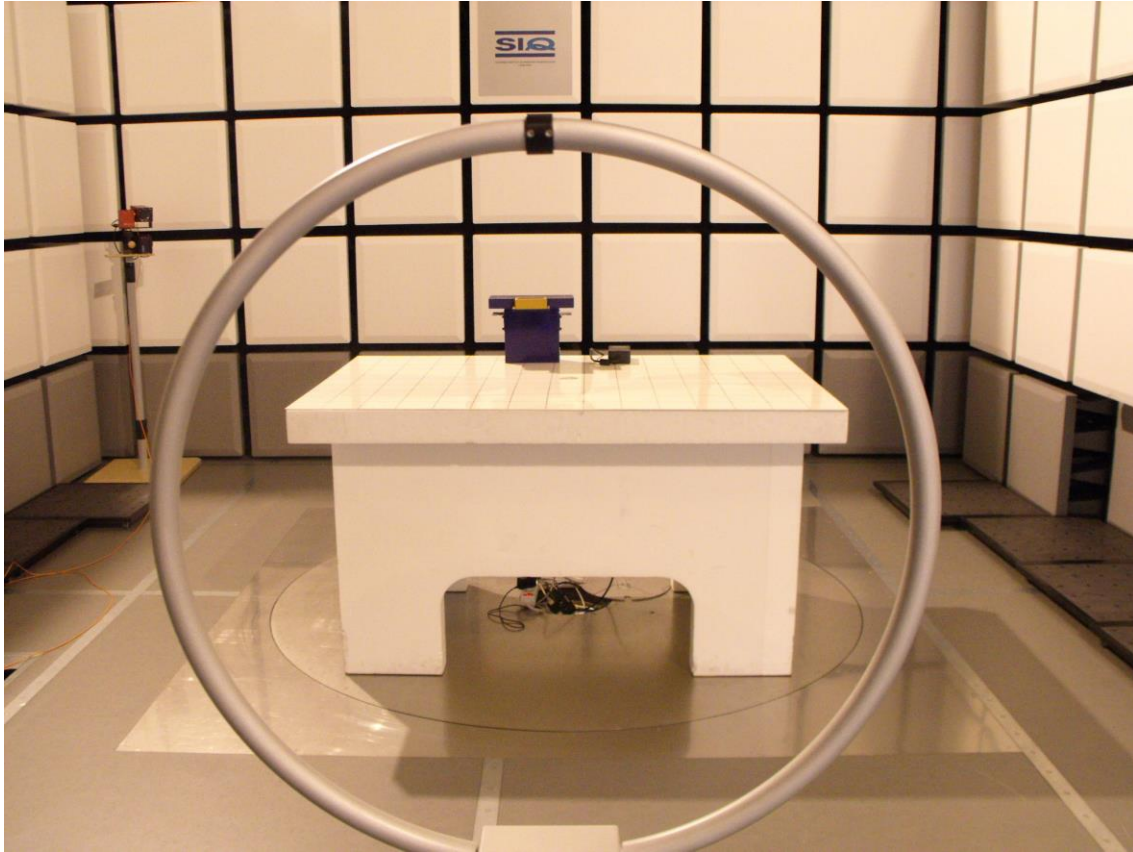
Figure 3: Radiated emission test from 9 kHz to 30 MHz
