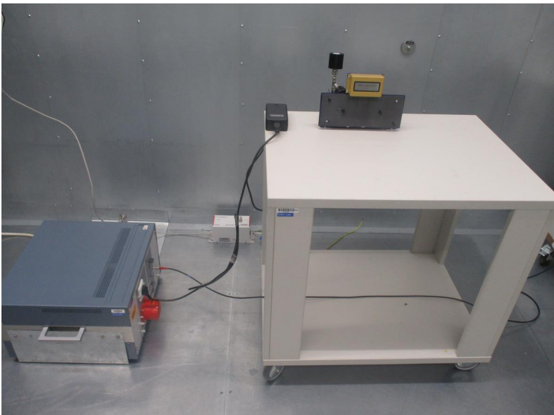
Figure 2: Conducted emission test with dummy load
