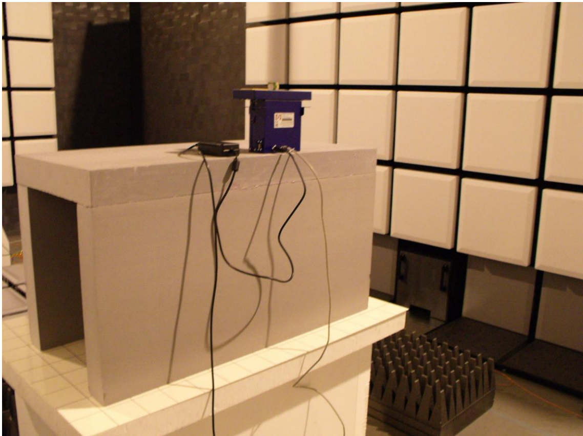
Figure 9: Radiated emission test from 1 GHz to 10 GHz
